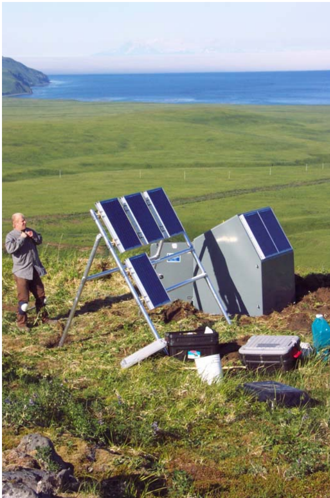
Figure 19: A telemetered geophysical station on Umnak Island recently installed by AVO, of the type to be employed for the Amchitka net. The geophone is buried in the ground and connected to the hut by a cable. The hut houses the GPS antenna and electronics for GPS, seismic, and telemetry. Power is supplied by solar cells. Such stations can operate unattended for up to 5 years. (Photo: S Moran, USGS). Equipment placement will take into account the strong winds.
