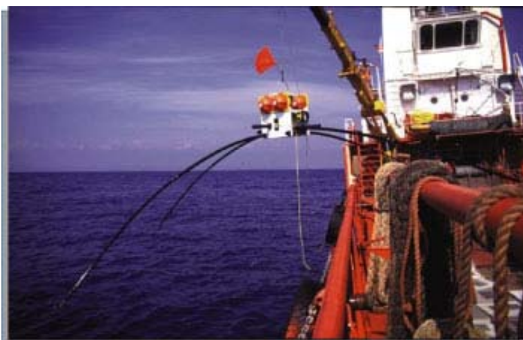
Figure 18b: Deploying offshore version of EM gear. Tips of the long poles contain the E-field electrodes.
