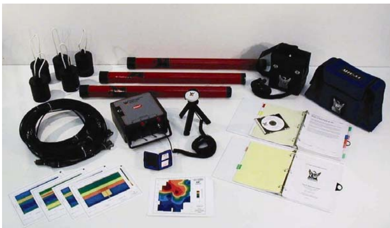
Figure 18a: From top left to right (5) E-field electrodes, (3) H-field sensors, battery pack, receiver case, cables, receiver, GPS antenna, software, electrical section plots, palm pilot IR receiver controller, plan view plots of resistivity. This equipment has been used throughout the world in all environments wet and dry, hot and cold.
