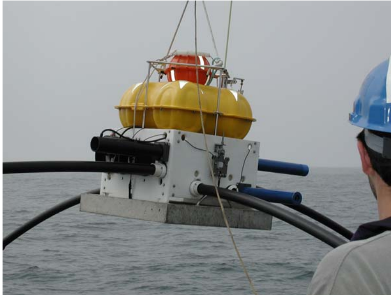
Figure 18c: Close up of the offshore EM gear. Blue rods are the H-field sensors, black rods spread the E-field electrodes, and yellow box contains the receiver.
